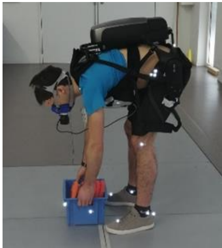
169 Figure 1. A subject wearing the ExoBack and all the measuring equipment.
