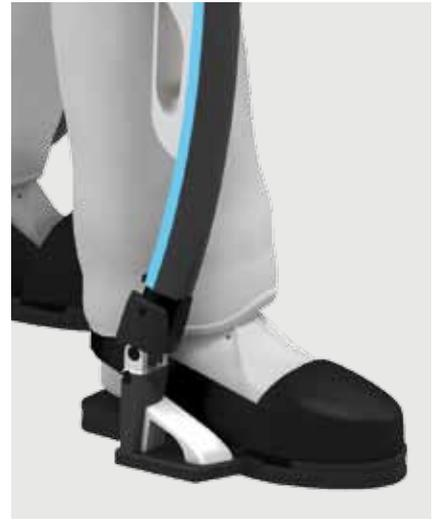
Flexible foot attachment system, for easier walking. RB3D patent.
