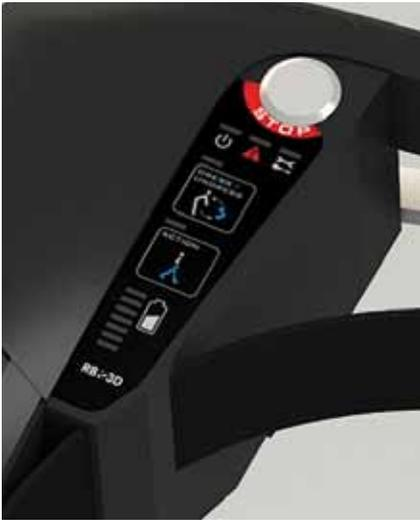
Ergonomical Human-machine interface on top of front platform.
